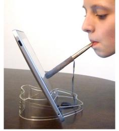
Figure 59: Examples of styluses and mouthsticks.
