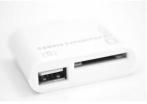
Figure 55: The iPad Camera USB Connection Kit.
